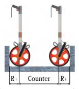
Place your Roto-Sure Measuring Wheel on the ground, with the back of your wheel up against the starting wall. Proceed to move in a straight line to the end wall, and stop the wheel up against it. Record the reading on the counter. The reading must now be added to the diameter of the wheel.
