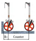
Place your Roto-Sure Measuring Wheel on the ground, with the back of your wheel up against the wall. Proceed to move in a straight line to the end point. Stop the wheel with the lowest point over the mark. Record the reading on the counter. The reading must now be added to the radius of the wheel.
