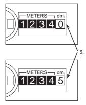
6. In the event that the counter does not read as indicated, there could be dirt or debris stuck in the timing belt. In order to correct this, please remove the timing belt cover and clean out any dirt or debris lodged between the teeth of the timing belt as well as the pulley.
