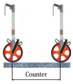
Place your Roto-Sure Measuring Wheel on the starting point of the measurement, with the lowest point of the wheel on the starting mark. Proceed to move in a straight line to the end point. Stop the wheel with the lowest point over the end mark. Record the reading on the counter. This is the final measurement between the two points
